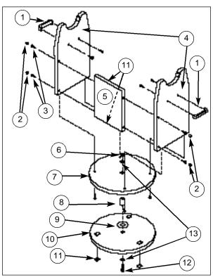
**Fig. 2:** Construction of the Dobsonian Mount. (1) Handle; (2) Screw Cover Caps; (3) Wood Screws; (4) Side Boards; (5) Front Board; (6) 5/16" Locking Nut; (7) Base Plate; (8) Center Bearing Bushing; (9) Nylon Washer; (10) Ground Plate; (11) Rubber Foot; (12) 2 14" x 5/16" Hex Pivot Bolt; (13) Flat Washers.
